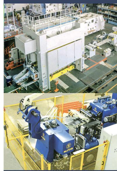
unique in that the automatic production line requires only two people to run. The high productivity is ensured by this rollingfeeder. Moreover, the metal thickness may be anywhere between 0.5 mm to 10 mm.
